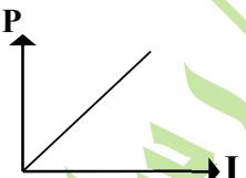
$$\begin{aligned} \therefore P &= \frac{E}{t} \\ \therefore E &= QV \\ \therefore Q &= It \\ \therefore P &= VI \end{aligned}$$
